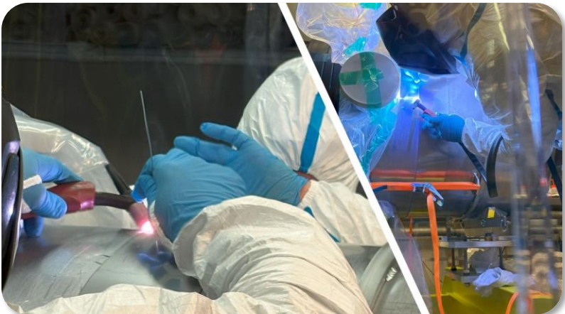
Tack welding in portable cleanroom
