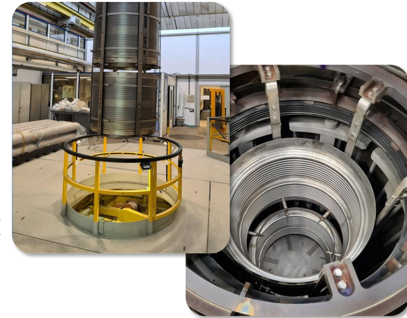
Vacuum firing of 304L bellows
