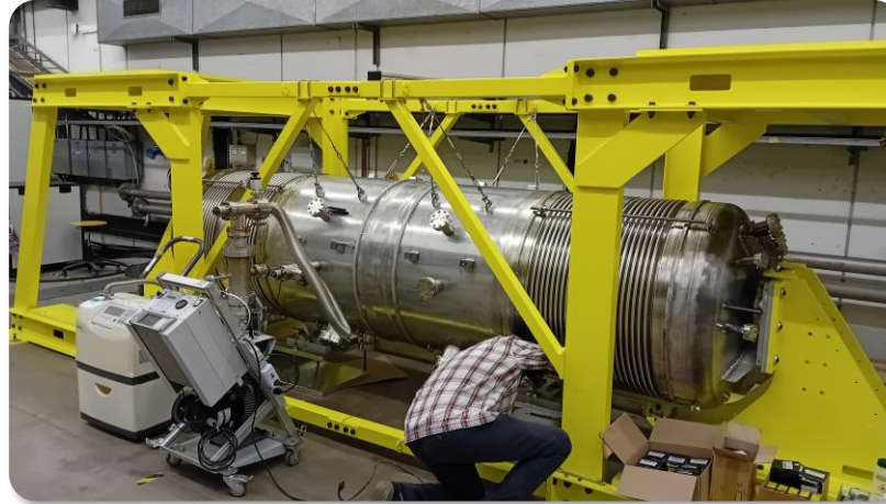
Bakeout and vacuum measurements on mock-up and preparation work for background test
