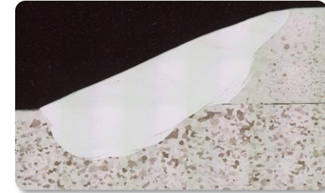
Fillet weld metallography
