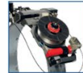
On-board wire feeder with straightening device
