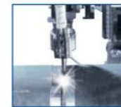
Torch module "V2 Narrow Gap", for wall thicknesses up to 75 mm
