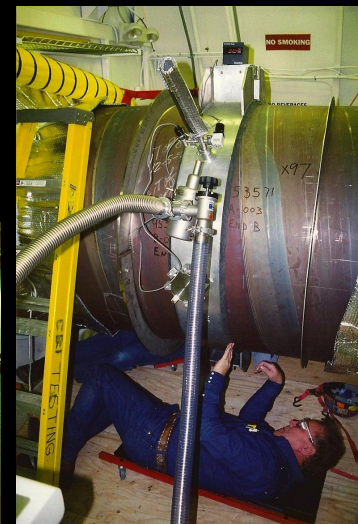
Field weld He leaktest (LIGO/CBI)
