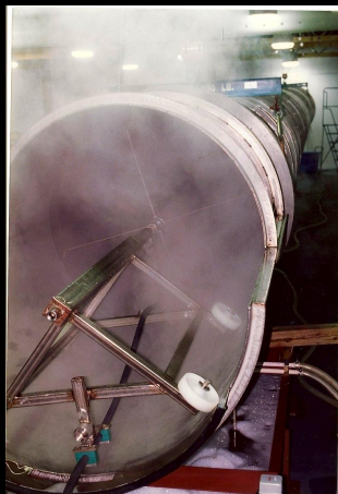
Detergent/hot water cleaning (LIGO/CBI)
