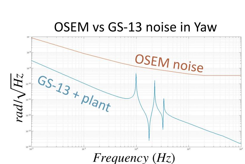
Motion of the suspension is the blue trace, which is, at the least, a factor of 5 below OSEM noise, making it difficult to get accurate measurements
