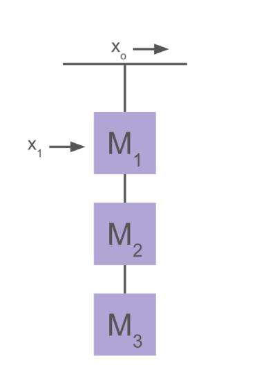
The OSEM measures the gap between the suspension point and the mass M1:  $gap = x_0 - x_1$
