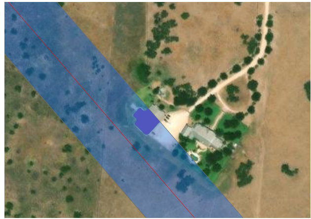
Figure 3. Successful test of a pre-trained building extraction model in ArcGIS Pro. The red line depicts part of the beam tube, while the translucent blue is part of the 50 m buffer. The building enclosed within the buffer extent is identified by the blue polygon.
