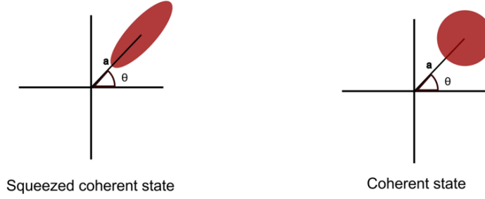
Figure 2: States of light in quadrature picture. The red area is the area of uncertainty of the state of light. Here r determines how much the squeezed and anti-squeezed quadratures are scaled. Both squeezed states here are phase squeezed because their uncertainty along the amplitude axis increases while the area along \theta is decreased.
