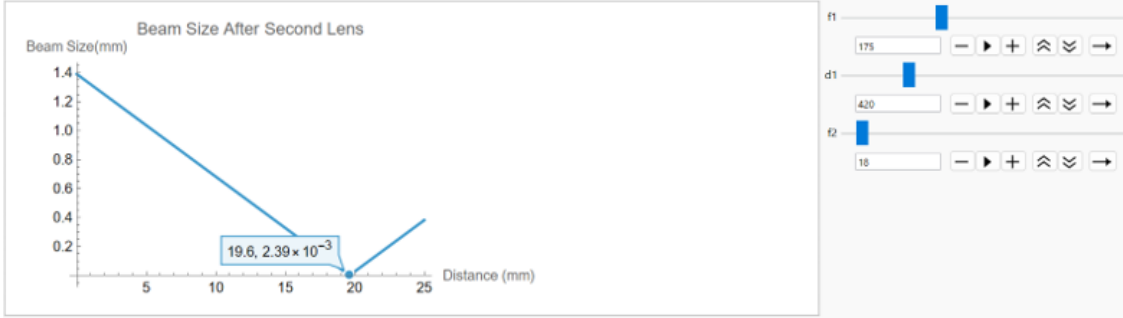
Figure 21: Lens solution for focal lengths of lenses ( f_1=175\text{mm} , f_2=18\text{mm} ) and distance between lenses ( d_1=420\text{mm} ). This lens combination allows for the beam to have a waist of 2.39\mu m , which is small enough for free space coupling into the crystal.
