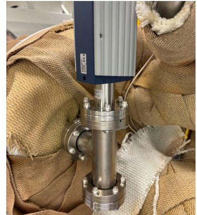
Figure 2.3-5 Tee-assembly of feedthrough and pressure gauge
