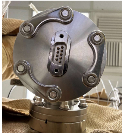
Figure 2.3-3 Underside view of feedthrough exposed to room air
