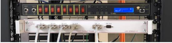
Figure 9: The chassis used to control the individual heater elements.
