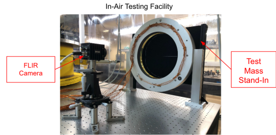
Figure 8: Testing setup of the Ring Heater, Test Mass substitute, and IR Camera.
