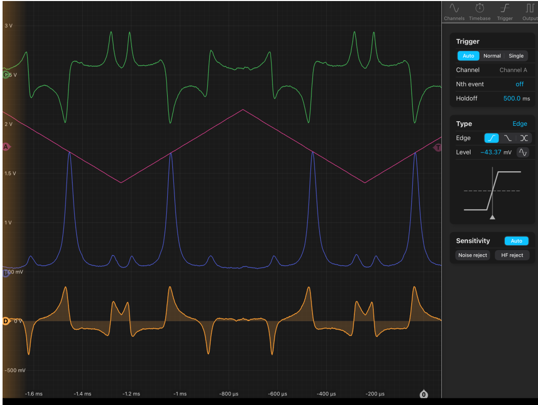
Figure 10.1: Transmission profile (blue) while driving the laser current (red) with a triangle wave to sweep laser frequency across cavity resonances. The PDH error signal (green) and known sideband modulation frequency lets us convert the x-axis to MHz. The yellow trace is the DC monitor on REFL PD.
