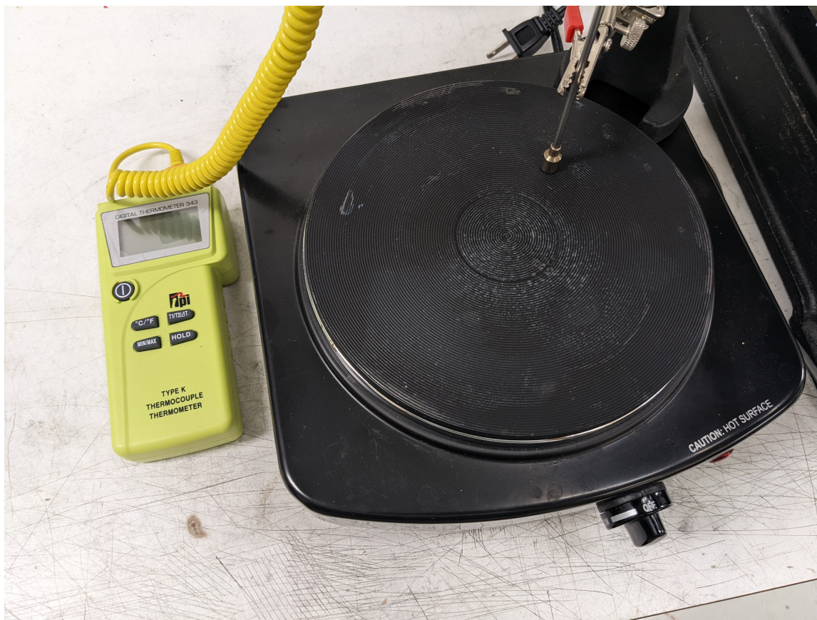
Figure 15: The Type K thermocouple was attached to the Digital Thermometer 343, and the measuring tip of the thermocouple was mounted parallel against the Oster hot plate. Per the thermometer manual, the tip must be held in place for at least 30 seconds to get an accurate reading.
