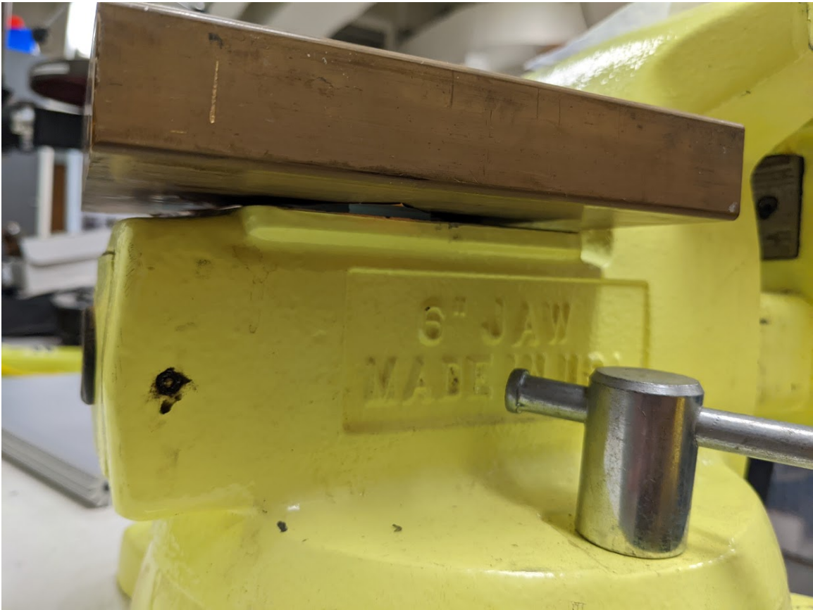
Figure 4: This is a bonded sample underneath the heavy brass mass. There is copper foil between the glass and metal to provide a buffer.
