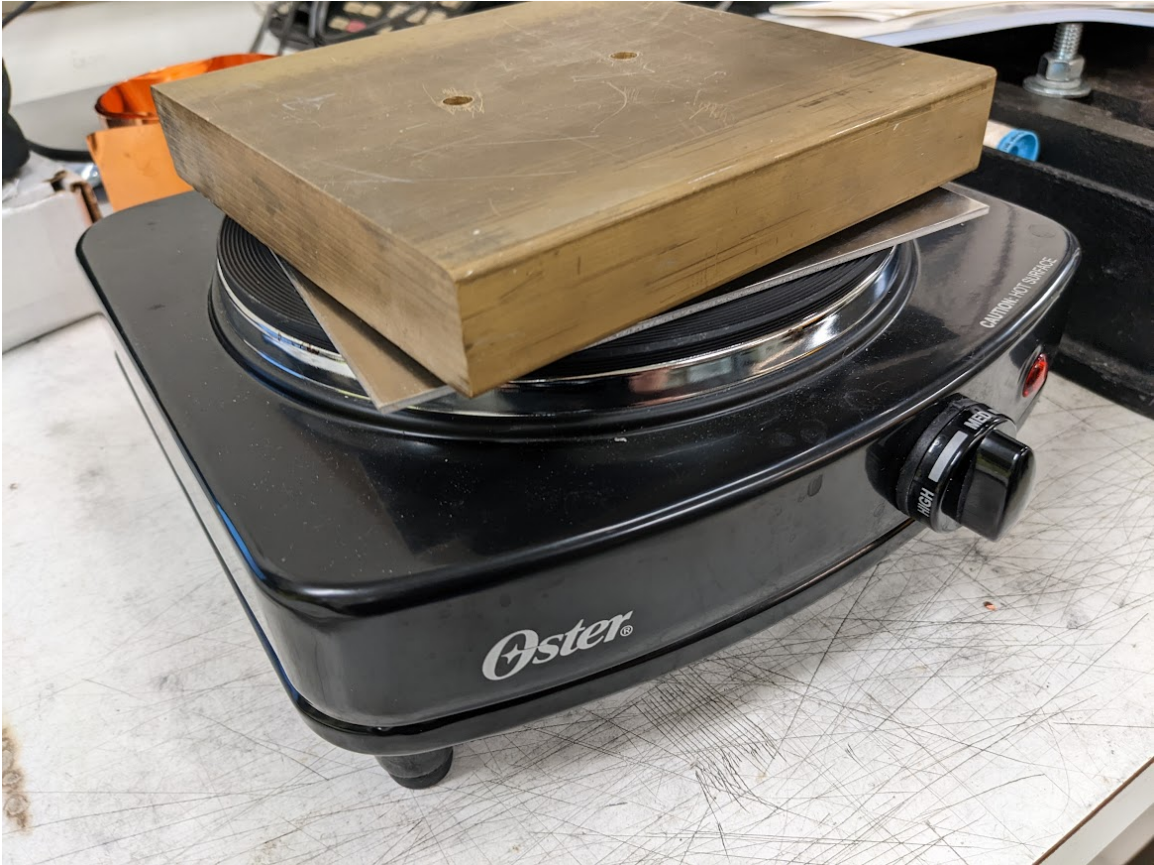
Figure 6: To heat a sample with pressure, I did the same as without pressure, but with a brass weight on top and copper at the metal-glass interface. I could not preheat this setup without risking burning my fingers.
