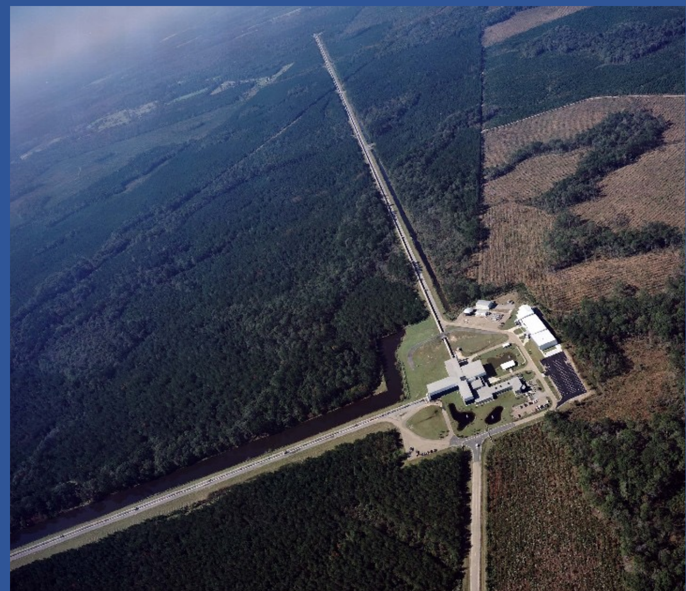
Fig. 1: The LIGO Livingston Observatory (left) in Louisiana and the LIGO Hanford Observatory (top) in Washington State. The arms of each site are 4 km (2.5 mi) long.
