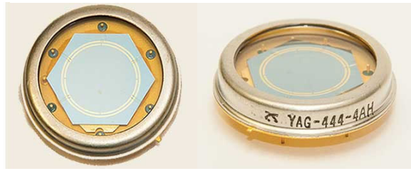
Figure 2 Excelitas YAG-444-4AH in a TO36 package
