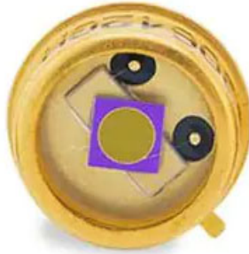
Figure 3 Excelitas C30642GH in a TO18 package
