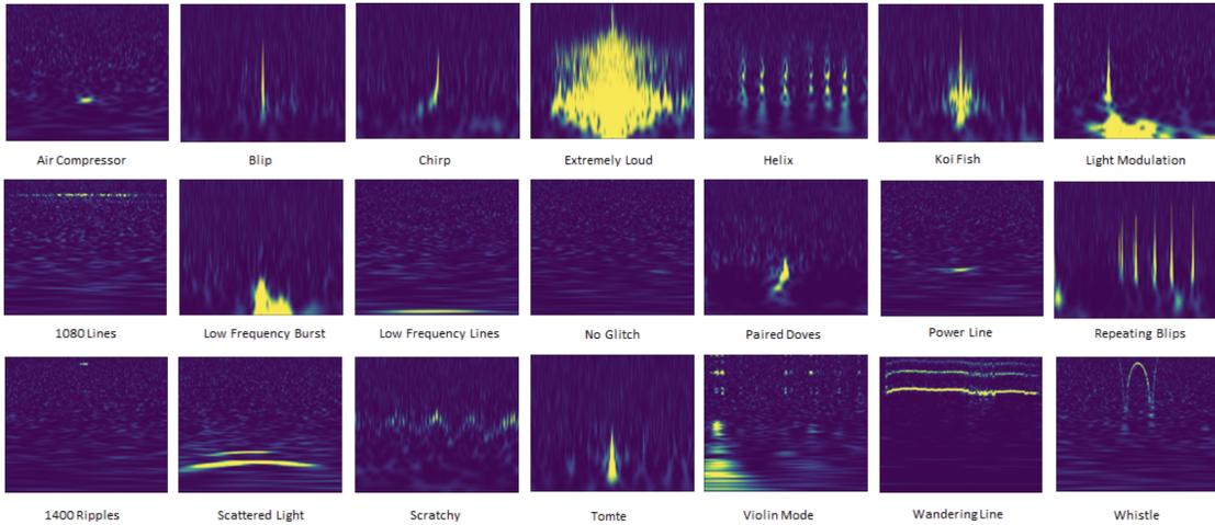
Figure 1: The figure, adapted from [3], depicts representative examples from 21 classes of glitches from the Gravity Spy Catalog [2] found in the strain data across the 3 observing runs of LIGO. The diversity in morphology across classes may hint towards various environmental and instrumental origins of these noise transients which result in false alarms in LIGO GW event search pipelines.
