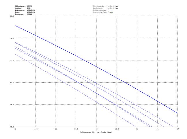
Calculated BS HR reflectance vs angle of incidence for various random 'designs' where the individual layer thicknesses have been slightly altered to simulate coating thickness errors. The perfect coating (exactly 50%) passes through the dot at 44.97 deg AOI.
