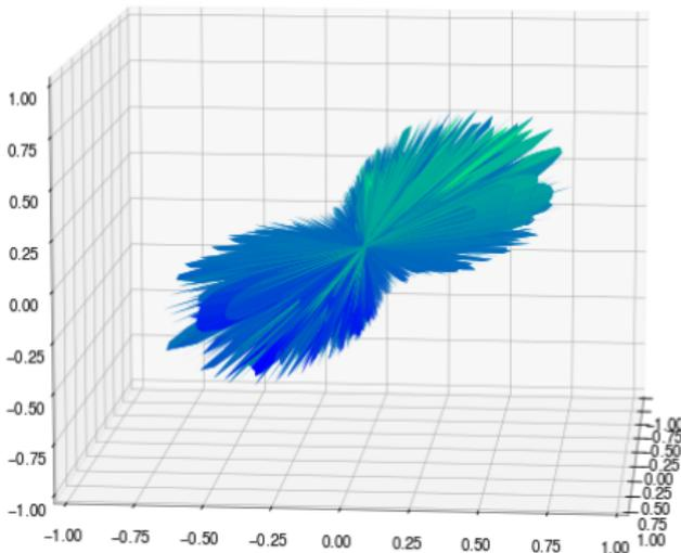
FIG. 7. 3D overlap function dependent on frequency at 1000 Hz. In this plot, the coloring aids in the 3D visualization and has no further significance. The axes represent the value of the overlap function at a given location.
