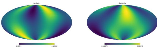
FIG. 3. The H1 cross (right) and plus (left) polarisation response functions. The dark blue and yellow represent locations in the sky in which the detector is most sensitive. The cross and plus polarisations allow for a wider range of high sensitivity.
