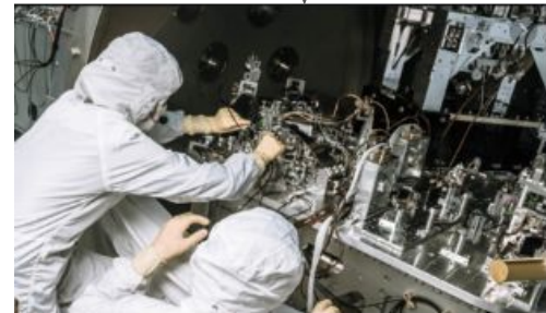
Optical system producing squeezed light to be injected in the detector
