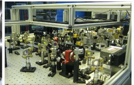
Optical system producing squeezed light to be injected in the detector
