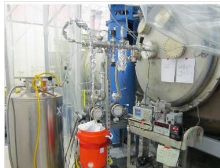
End mirror discharging system
