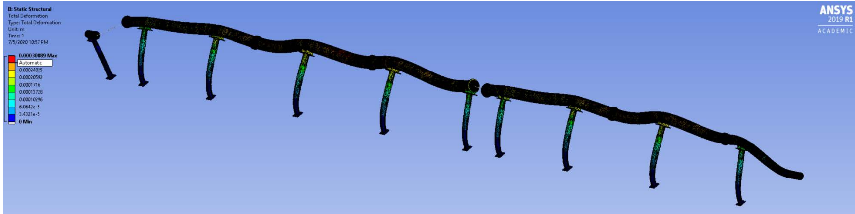
Figure 10 Gravitational load and lateral seismic, static-equivalent load
