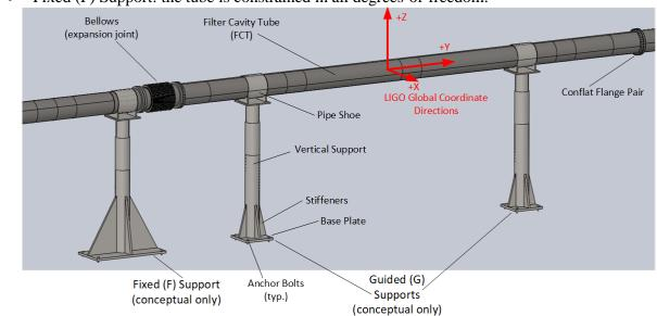
Figure 1 A representative section of the FCT (conceptual only)
