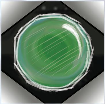
Optics are found throughout LIGO's interferometer. For example, at the end of each arm, a 40 kg (88lb) ultra-pure fused silica mirror reflects the laser light back down the arm.
