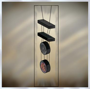
LIGO's mirrors are located at the bottom of four stages of a pendulum. This quadruple pendulum system greatly reduces the movement of the mirrors.
