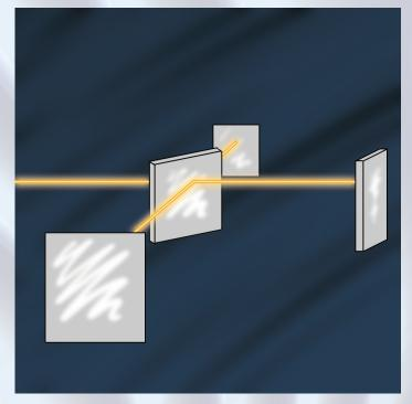
At the heart of LIGO's detectors is interference between the laser light that returns from each arm. Without a passing wave, the light signals cancel each other out. As a gravitational wave passes, the interference pattern shifts, signaling changes in the lengths of the arms.
