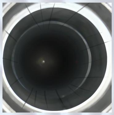
LIGO's needs ultra-high (10<sup>-9</sup> torr) vacuum to operate. To achieve this vacuum 10,000 cubic meters (353,000 cubic feet) of air were pumped out.
