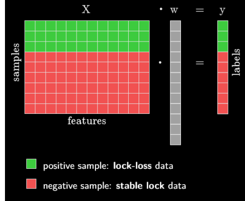
Figure 1: The Lasso regression attempts to solve for \mathbf{w} in this equation. Graphic courtesy of Rollins. 3
