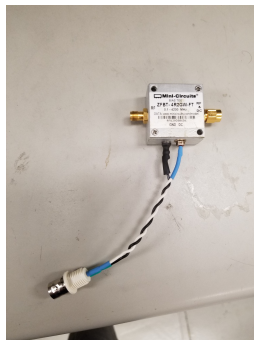
Figure 3: Bias Tee with Soldered BNC connector
