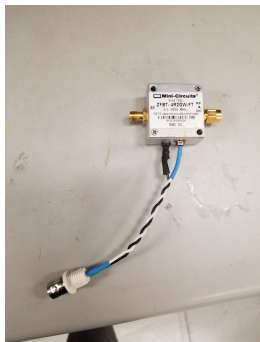
Figure: Bias Tee (Model ZFBT-4R2GW-FT) with Soldered BNC connector / Transfer Functions of Bias Tee in Regular Use
