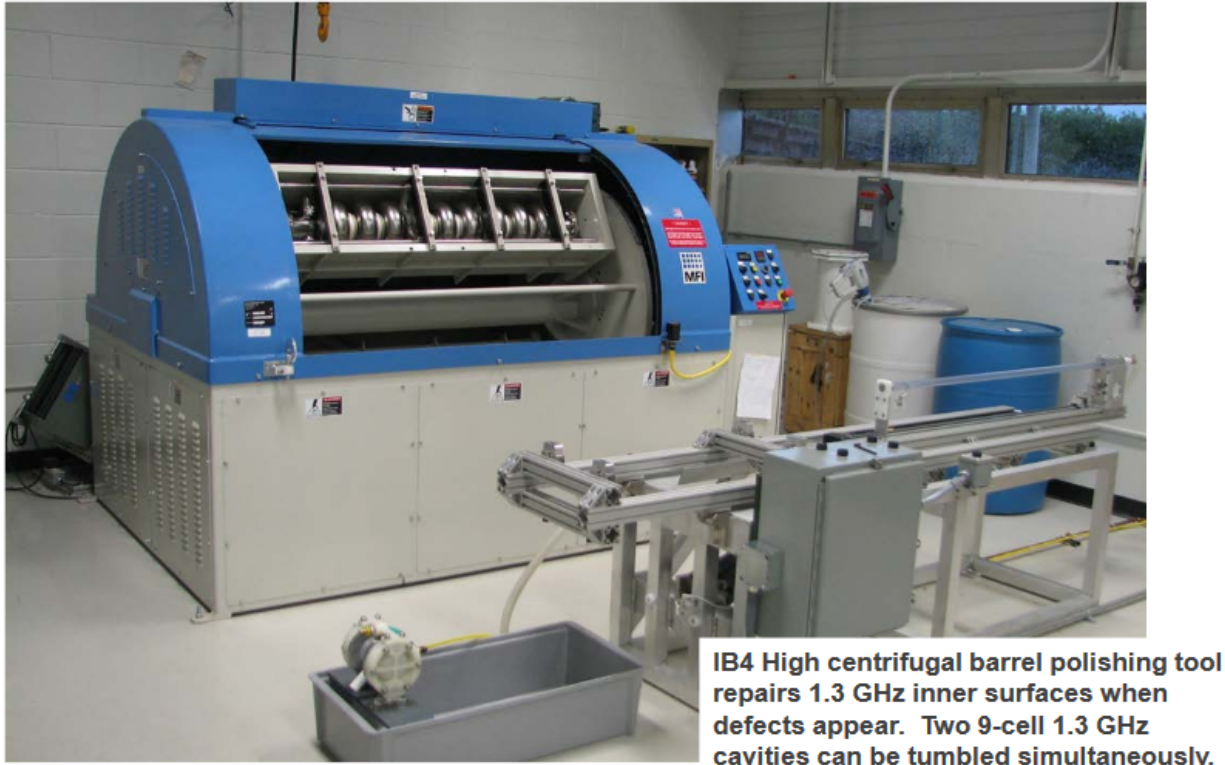
Figure 4: Barrel Polishing Setup (courtesy A. Rowe, FNAL)
