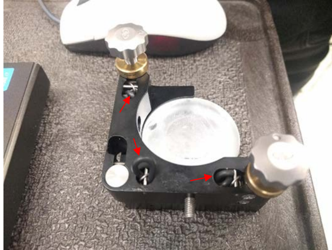
Figure 2: Viton O-Rings being pushed up against the springs in the mirror mount
