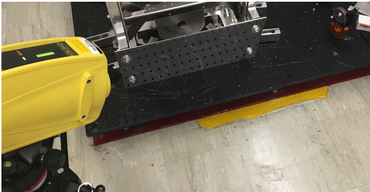
Figure 5: Experimental set up, highlighting the vibrometer axis used during testing
