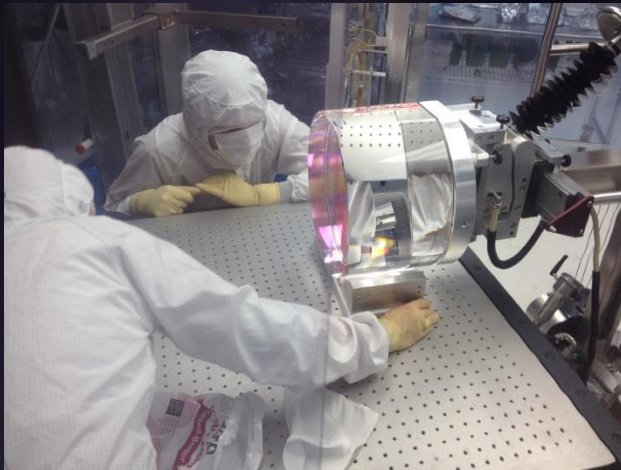
Large 40 kg mirrors with highly reflecting coatings
