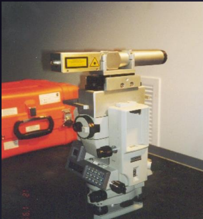
Infrared Laser Autocollimator (4W fiber coupled laser and Davidson D-271-106)
