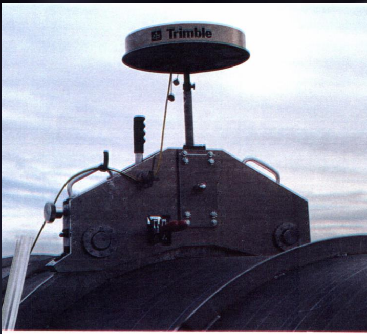
GPS Antenna Mounted on Beam Tube Support Ring (1997)
