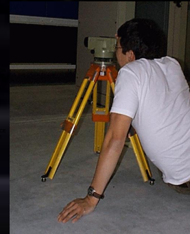
2. Tables positioned and aligned using "Total Station" Theodolite & Optical Level
