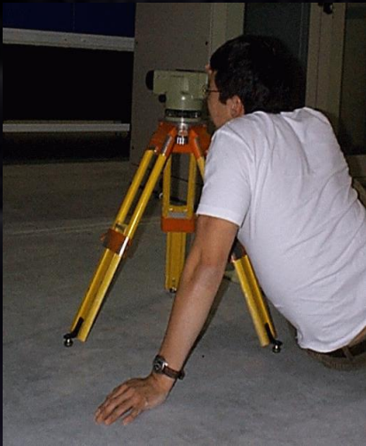
Optical level (Sokkia B2o AutoLevel)
