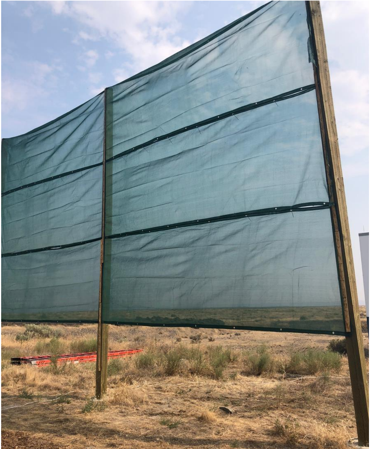
Figure 17: Prototype Wind Fence (Improved 50% Porosity Material)
