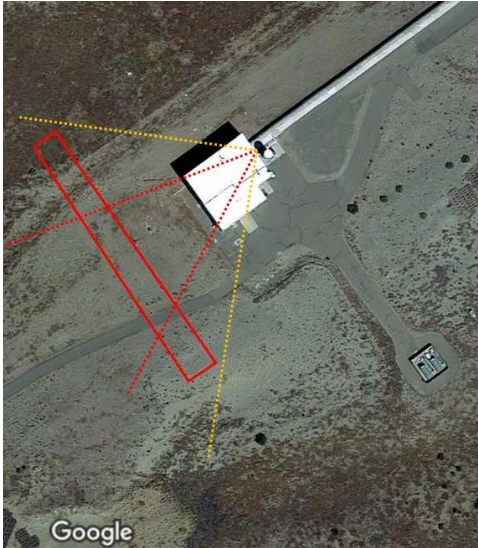
Figure 12: Sketch of different Wind Fence coverage cases at End Y Figure 12 Source: Q&A - LHO Wind Fence Design and Construction
