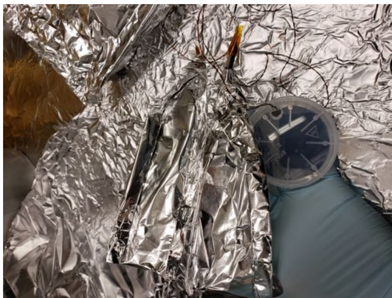
Figure 7: The three resistance temperature detector probes, and a fourth tester probe, prepared for calibration baths by sealing in foil. One of the RTDs is attached in between two sample silicon disks. To ensure that the disk surfaces would not be scratched, I modified a plastic wafer container to accommodate for the wire. Once sealed in foil, they were inserted into plastic bags.
