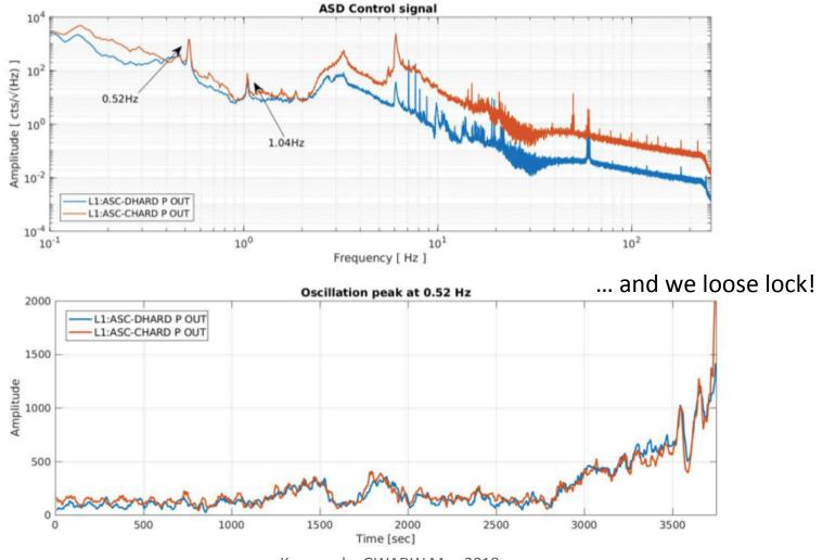
0.5 Hz soft radiation pressure oscillation:
