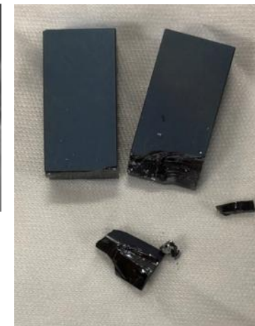
Silicon halves after bond strength test.
