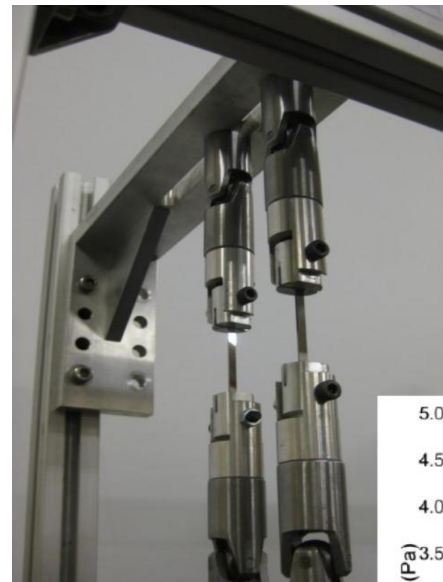
Strength tests on silicon ribbons etched from a wafer
