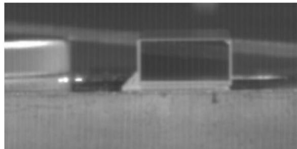
Thermal image through silicon sample to assess bond quality
