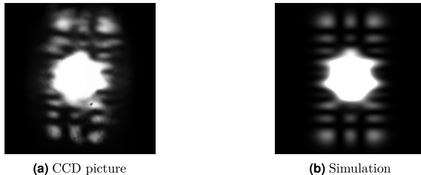
Figure 3.14: Output mode of the damaged OPA. After about four years of operation, the OPA showed a deformed mode shape with a clear TEM_{29} contribution. The left panel is a CCD picture of the beam exiting the OPA. The right panel is a qualitative simulation showing how scattering into higher-order modes inside the cavity can lead to a comparable beam shape if eleventh-order modes are co-resonant with the fundamental. The picture used an uncalibrated CCD and is intentionally overexposed in the centre in order to better resolve the outer mode shape. In a separate measurement it was determined that the higher-order modes made up about 8% of the total beam power.
