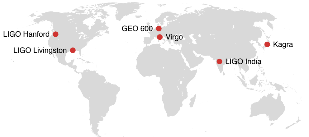
Figure 1.5: A map of the second-generation gravitational-wave detector network. GEO 600, Virgo and the two LIGO detectors are currently operational, KAGRA is under construction, and LIGO India is planned. Combined detections by as many detectors as possible distributed around the globe help with localizing the source of the signal in the sky.
