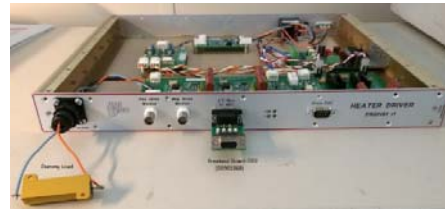
Figure 2 shows the dummy load, 75\Omega , connected to the heater driver output, CPC connector, label as “to SR3 Heater”. Also the breakout board –DB9 (D0901868) is seen connected to the “I/V Monitor to ADC”.
