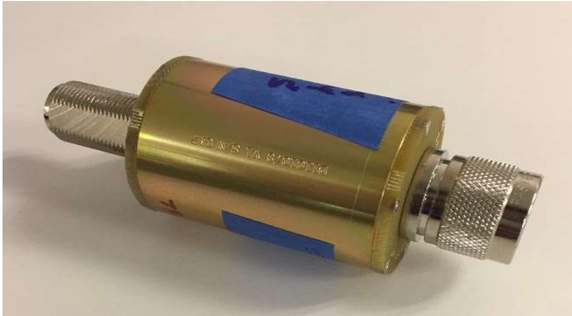
Figure 1a: DC ground isolation unit, or balun
