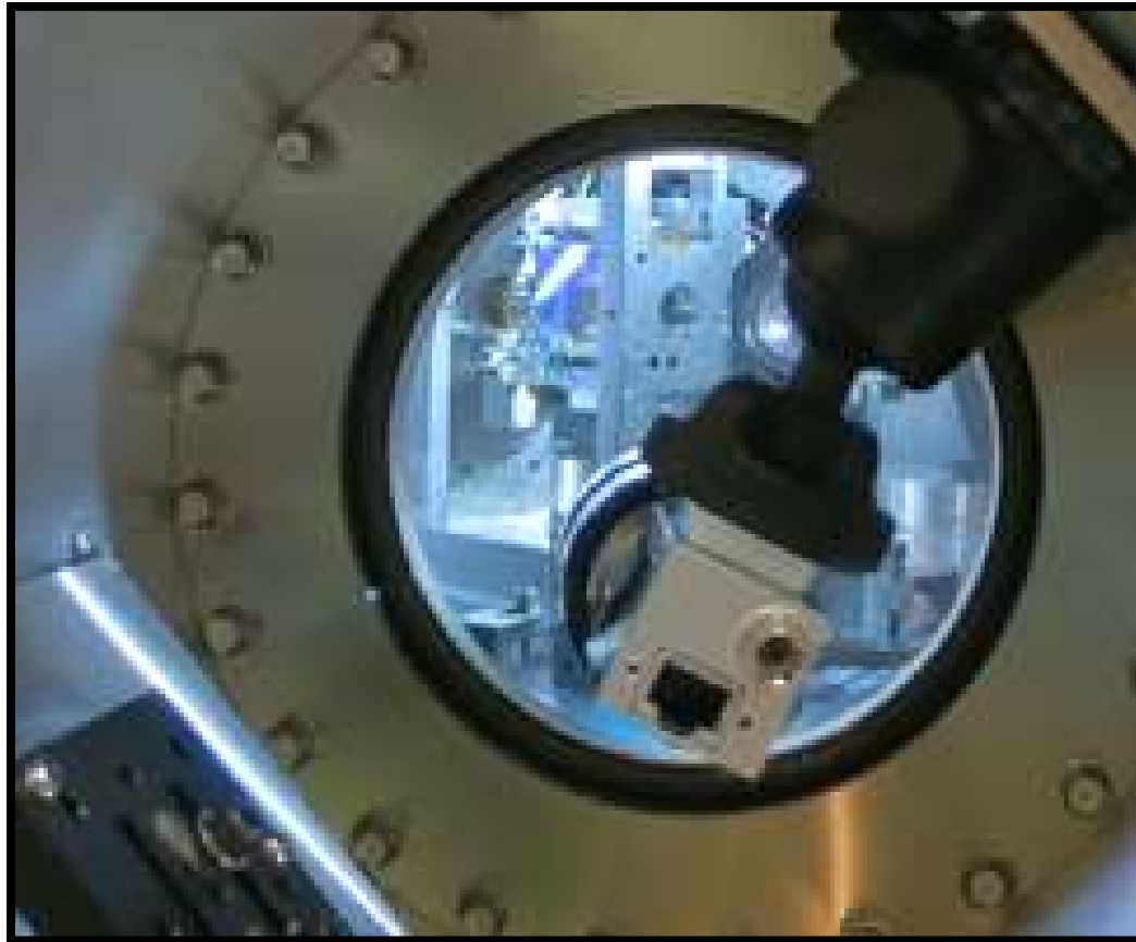
Camera installed at the viewport
