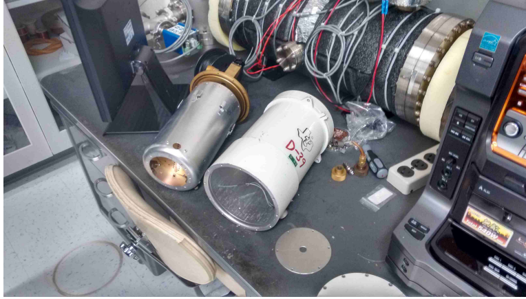
Figure 1: Cryostat with a work plate at the bottom that will be used to measure the heat flow across different sample interfaces.
