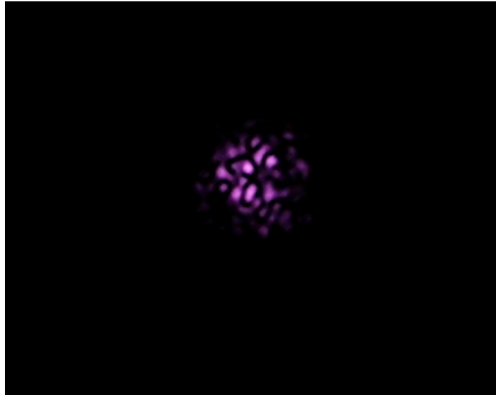
Figure 15: Image of stored beam interacting with coated reflector at the LIGO Caltech 40 Meter Prototype site.
