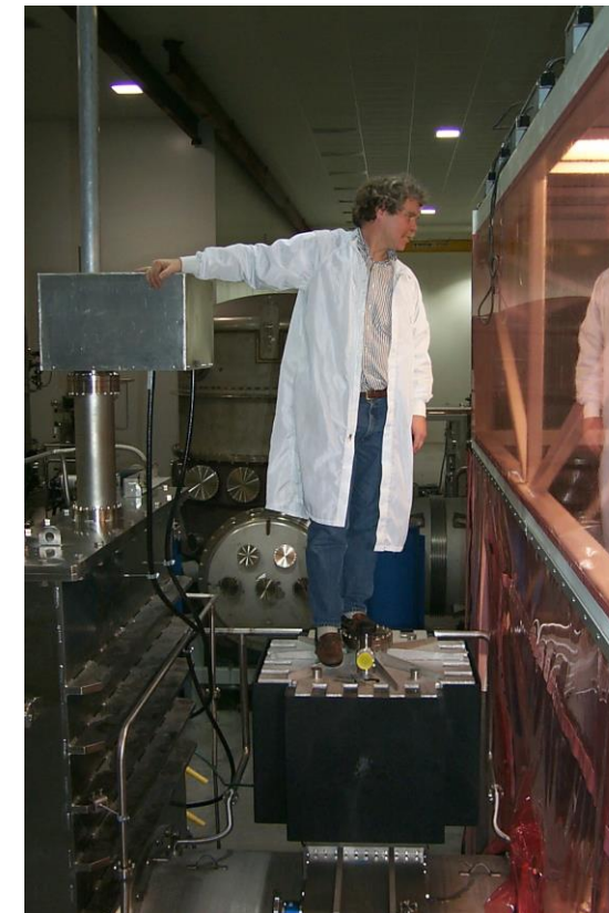
2500 l/s ion pumps (16.5" Conflat flange) with Ta "Noble Diode" Cathode
