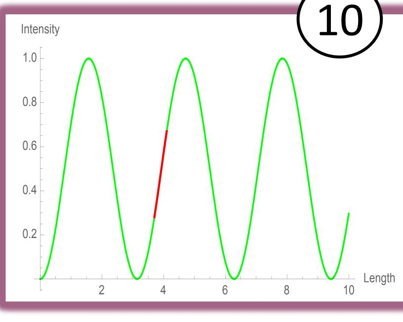
10. We will use a piezo in the interferometer to find the working point, i.e. the length at which the laser output is half of its maximum intensity. This will give the largest and most linear modulation induced by the effective length changes caused by the oscillating coated membrane.
