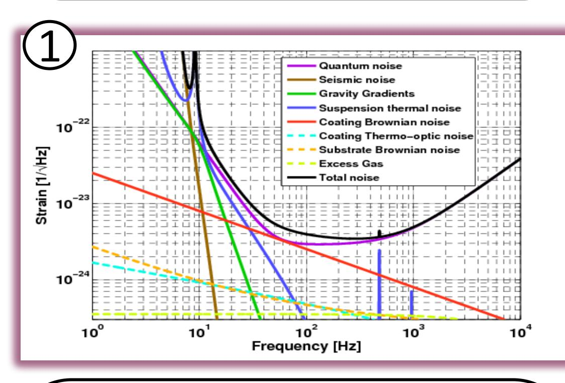
4. All resonant systems have an intrinsic Quality Factor (Q) that describes how rapidly they exchange energy with the thermal bath. A system with a high Q has low thermal noise.  $W_{Thermal} = \frac{kT f}{o}$
