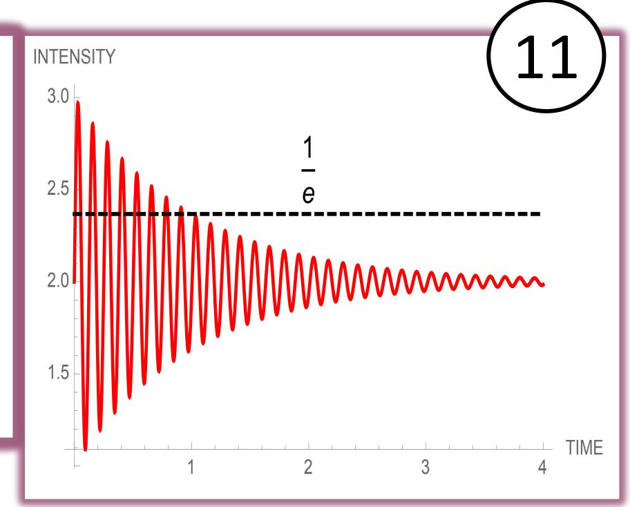
11. This is an example of the type of ring-down we will be measuring to calculate the Q value of the coatings.
