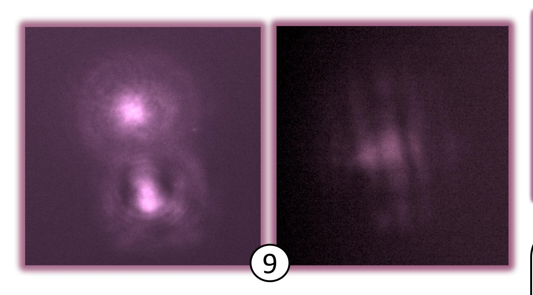
9. Work in progress: Our interferometer outputs two beams that, when aligned, show the interference pattern we will measure. We will need to design a photo detector that can accurately read the change in intensity as the fringes move across it, due to the oscillation in effective cavity length.
