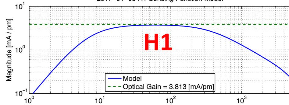
The modeled optical gain is about  $\sim 3.7$  [mA / pm] for both observatories (and remember, measurement matches our model very well).
