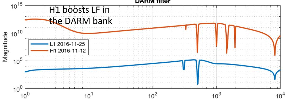
Digital gains (and a sign) are distributed differently on the sensing side, so DARM filter gain and sign compensate, otherwise pretty similar...
