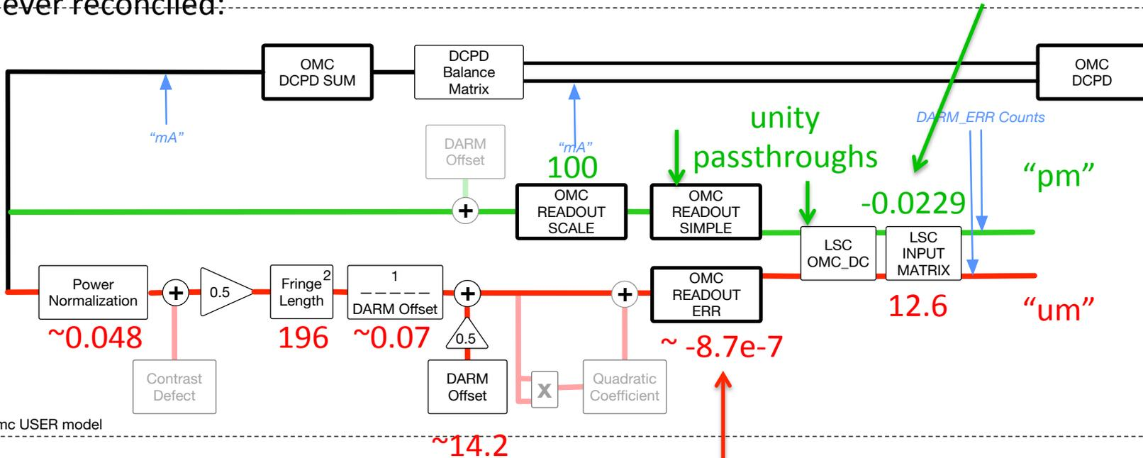
This gain factor is such that the OMC DCPD error signal matches the AS AIR, and AS AIR error is matched to ALS DIFF, which was originally (roughly) calibrated in “um”
