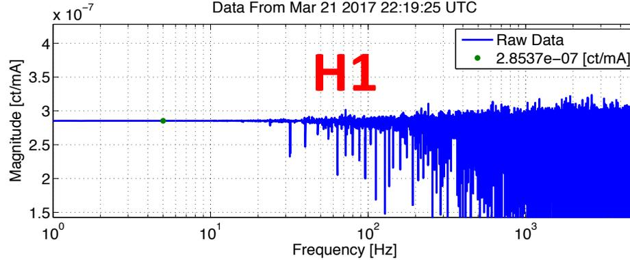
This explains the difference between the site's transfer function between the OMC DCPD SUMM (in [mA]) and DARM\_IN1 (i.e DARM\_ERR in [ct])
