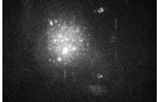
Figure 1. November 2015 Photograph of an End Test Mass at LIGO Hanford with an exposure time of 1.3 seconds. Crowding in the image is solely due to the finite size and nature of the Airy disks. The actual scatterers are expected to be of sub-micron size and widely separated within the actual coating layers of the End Test Mass. (Note: The rings and faint straight lines that appear in the background on the right side of the image are components of the mirror support structure).
