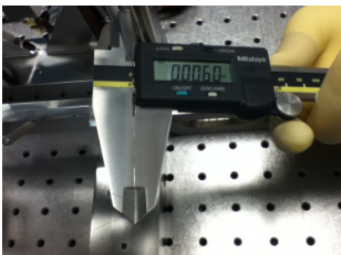
Measuring lower wire diameter
