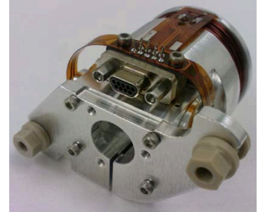
A BOSEM and its electronics
