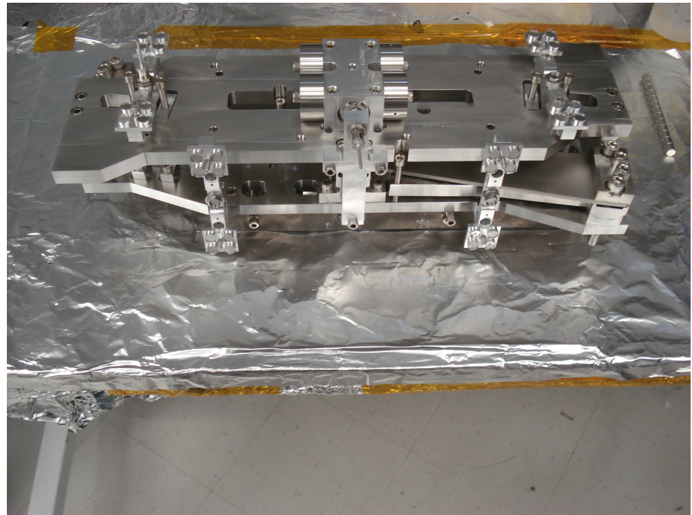
Quad top mass complete assembly
