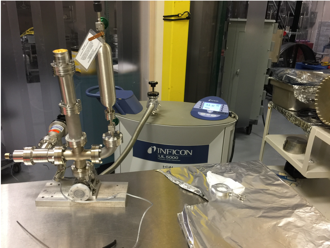
Fig 4: Leak Checking RGA Manifold
