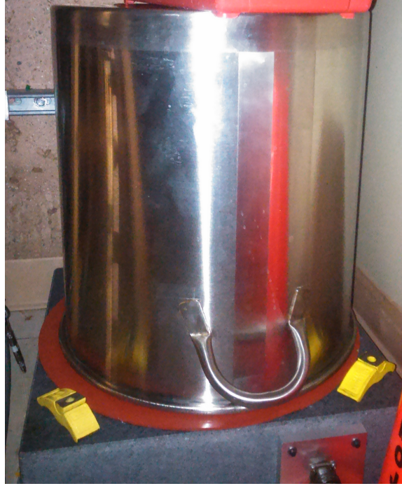
Figure 4: Photograph of Existing Enclosure for seismometer
