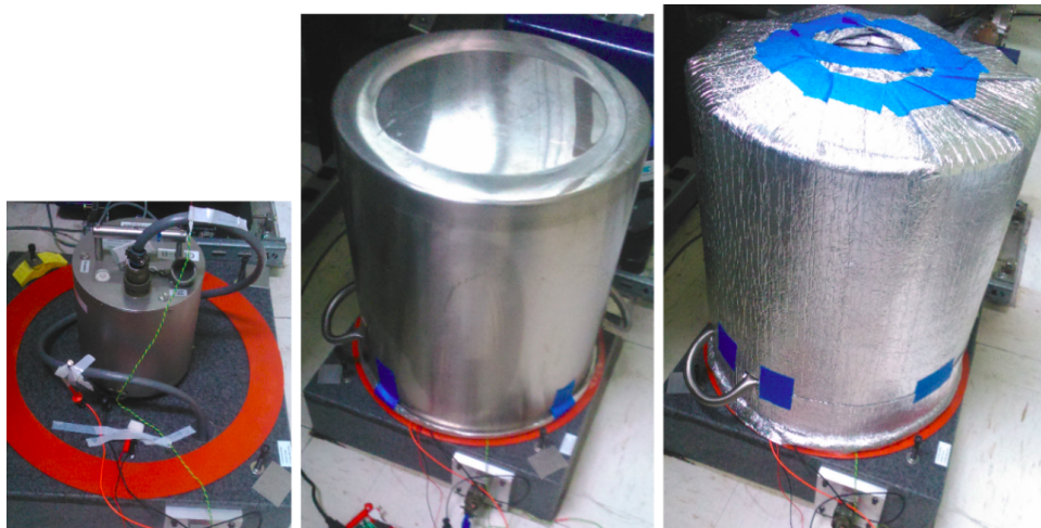
Figure 13: The seismometer, existing enclosure and enclosure with insulation
