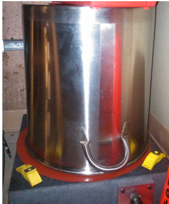
Figure 8: Photograph of Existing Enclosure for seismometer
