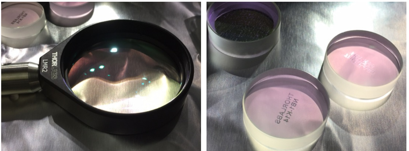
Figures 7 and 8: A clean lens(left) and the three clean mirrors (right) following the First Contact procedure.
