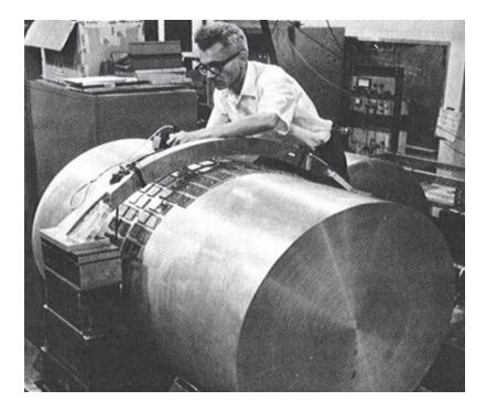
Weber's gravitational wave detector was a cylinder of aluminum. Each end is like a test mass, while the center is like a spring. PZT's around the midline are Bondi's dashpots, absorbing energy to send to an electrical amplifier.
