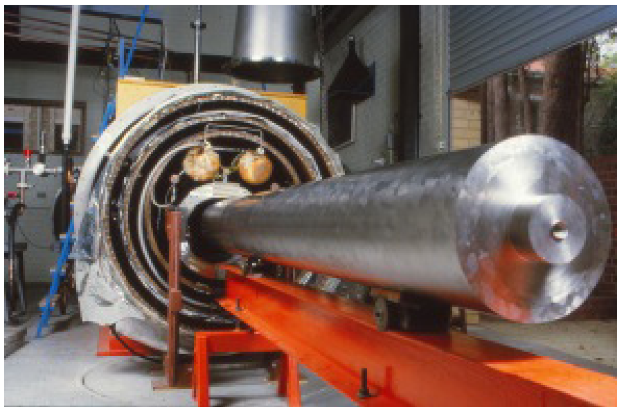
Fig. 1.6 a) The AURIGA aluminium bar that was cooled below 100mK and used a SQUID passive transducer, and b) the NIOBE detector, made from niobium, with a microwave parametric transducer.
