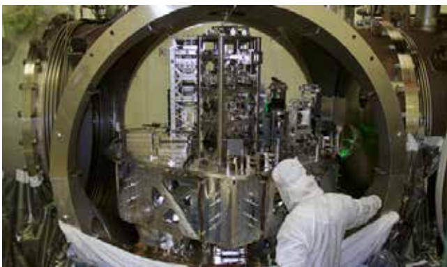
Small optical systems suspended inside a LIGO vacuum chamber.
