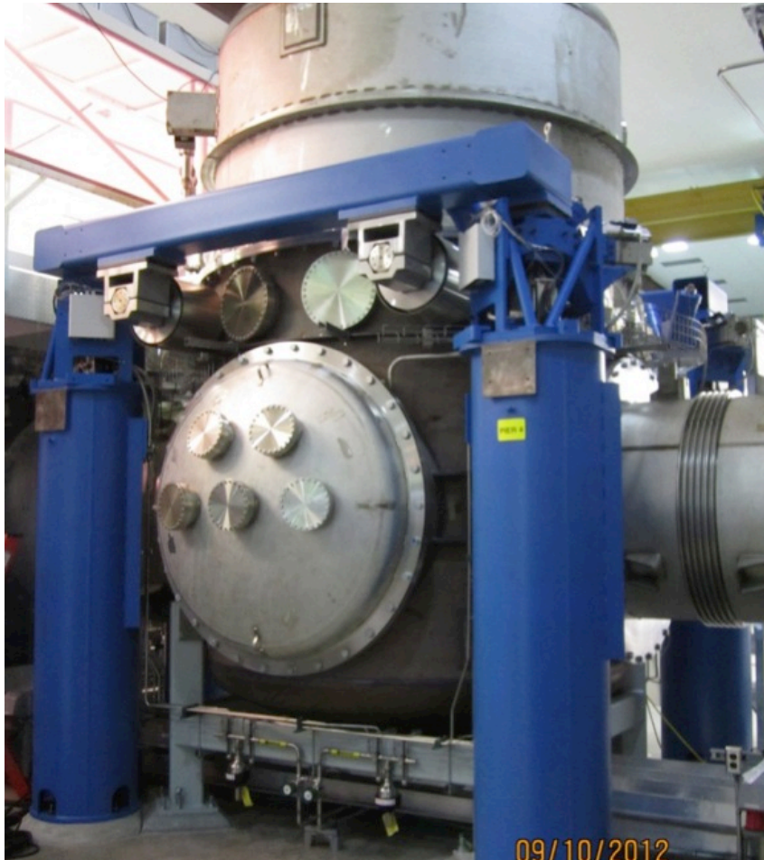
hydraulic external pre-isolator (HEPI) (one stage of isolation)
