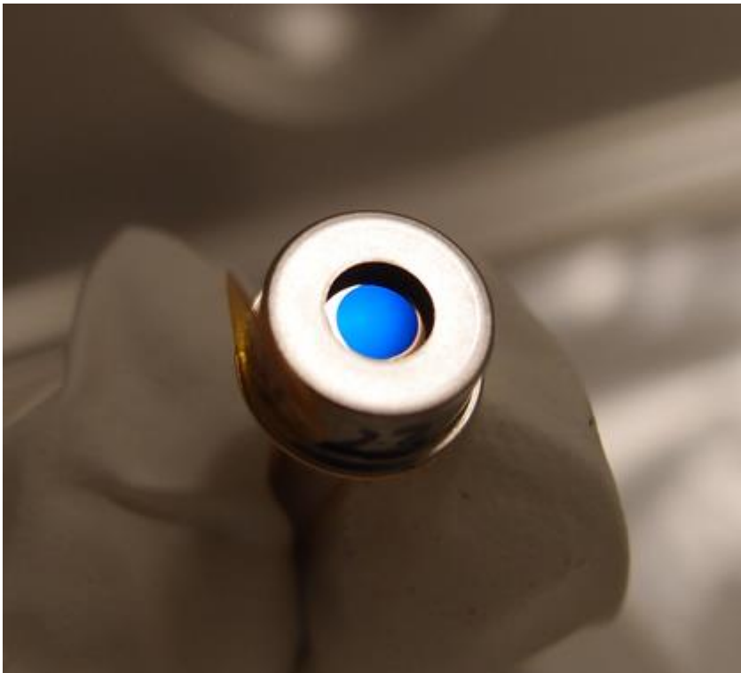
Figure 5: IGHQEX3000 InGaAs Photodiode with seal removed
