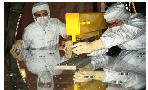
Deinstallation of an Initial LIGO seismic isolation platform at LHO.
